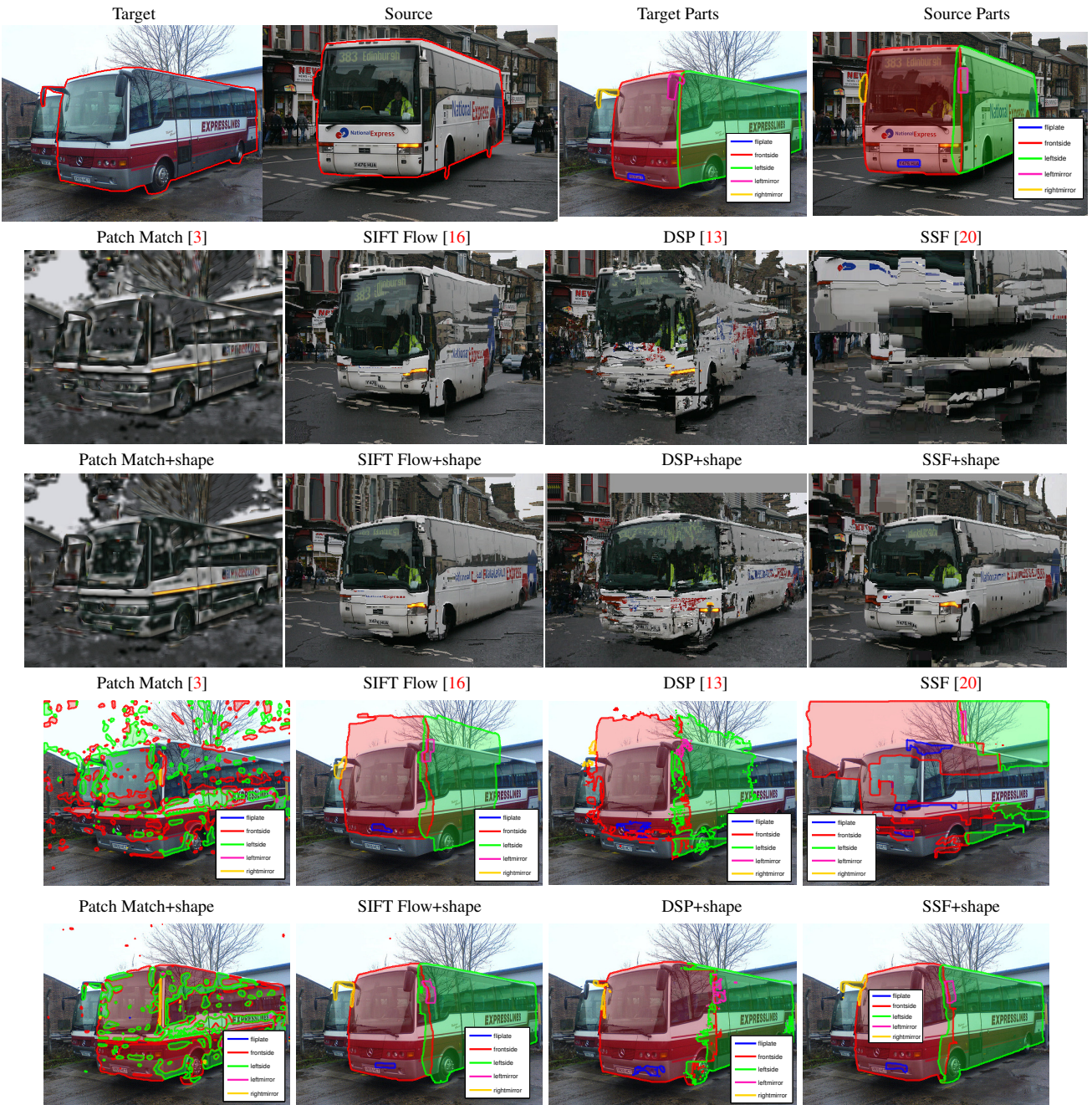
Figure 5: A qualitative result from the PASCAL-Part dataset [6]. First row shows the target and source images with ground truth segmentations marked in red along with the target and source image part masks. Second and third row show the warped source image using the default settings and with shape constraints respectively. The expectation is that the warped source image reconstructs the target image with the appearance of the source image. The fourth and fifth row show the part mask transfer from the source image to the target image using the default settings and with shape constraints respectively. Ideally, the part masks transferred from the source image should coincide with the part masks of the target image. See also supplementary material.
